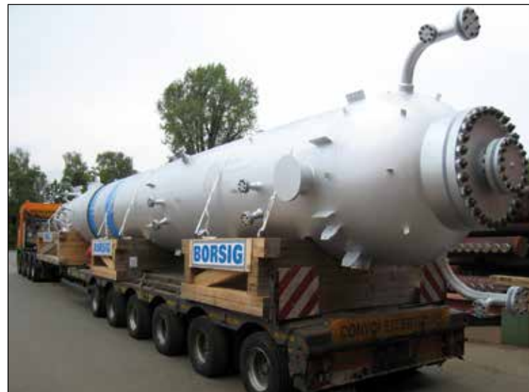
BORSIG synthesis gas cooler downstream of partial oxidation
