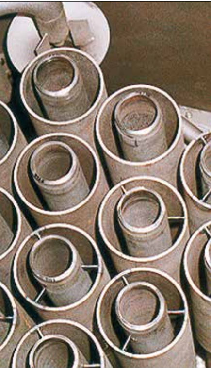
Assembly of connecting pipes and double tubes
