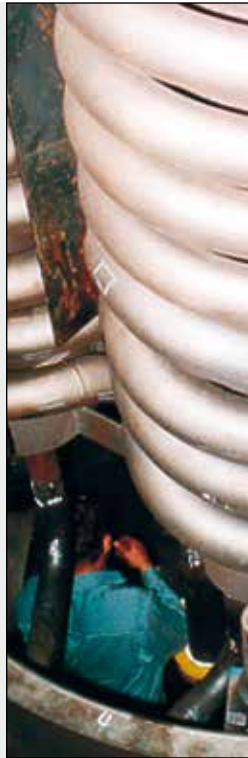
Spirally wound heating surfaces
