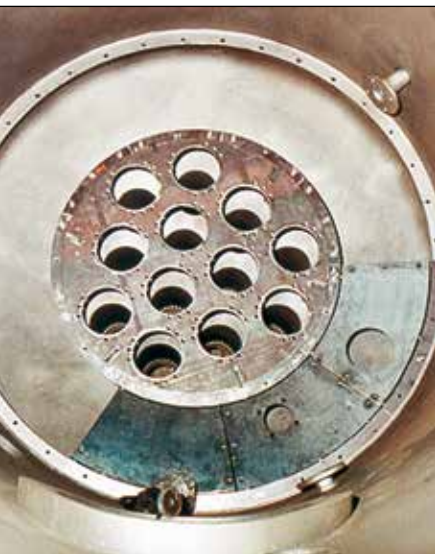
Assembly of connecting pipes and double tubes
