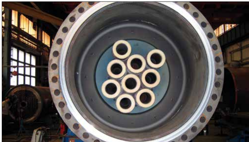
Inlet section with nozzles syngas cooler (TEXACO/GE)
