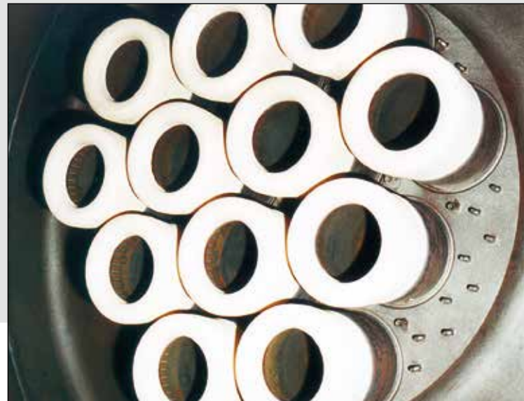
Ceramic coating of the gas inlet nozzles
